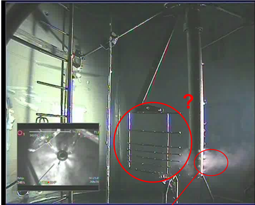
Sparger experiment in the PPOOLEX facility. SPA-T6, low steam injection phase
