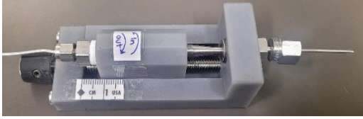
Fig. 2. Thermocouple probe radial adjustor.
