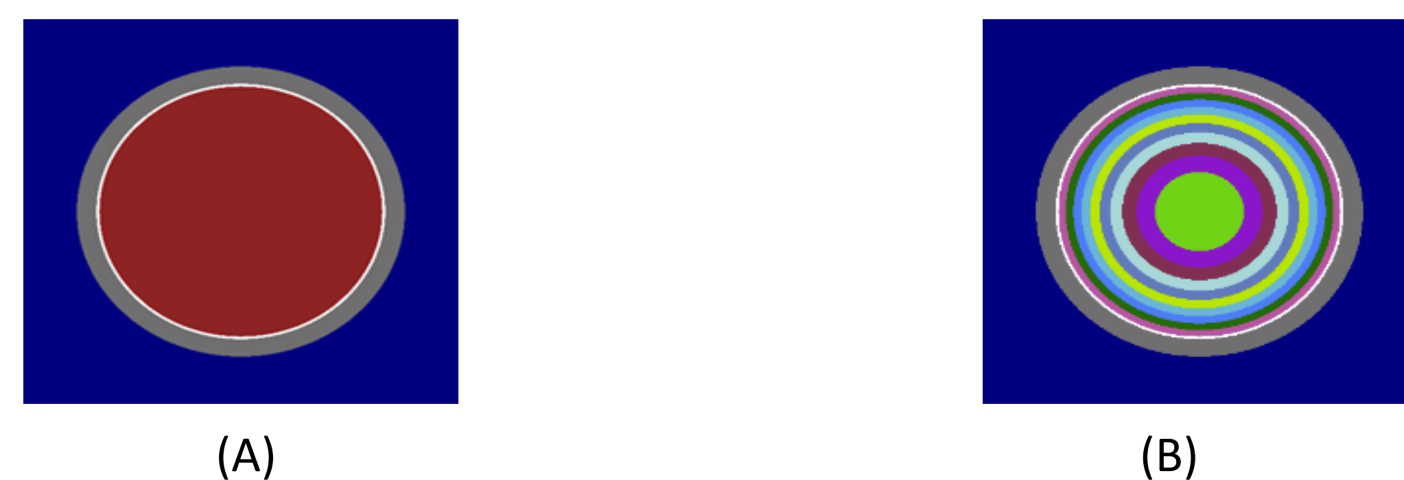
Fig.1. Westinghouse 17 × 17 PWR pin cell model (A), fuel-cladding system with fuel region divided into 10 rings (B).
